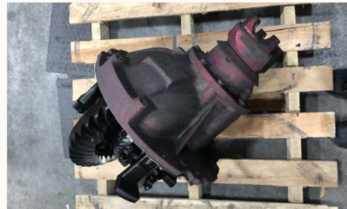
Engine 21 differential replacement
